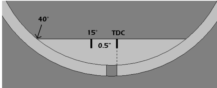
There is a flange at the bottom of the inspection cover opening. Beneath the flange is a notch in the case. Make a mark on the flange directly above the right side of the notch. This will be your Top Dead Center mark. Make another mark 0.5 inches to the left of the TDC mark. This is the 15° initial timing mark which is equivalent to the "F" mark on breaker point bikes, and the "Π" mark on TCI bikes. The 40° total advance point is on the left side where the flange meets the case.
